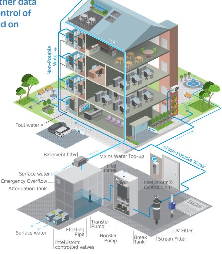
SDS WaterBank® Intellistorm® maximises the capacity for water reuse utilising only the attenuation volume, whilst minimising the potential for flooding by controlling the discharge of excess stored rainwater prior to a rainfall event.
